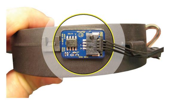
2. Lower the fan into the rear housing. Press the foam gasket into place across the top of the
